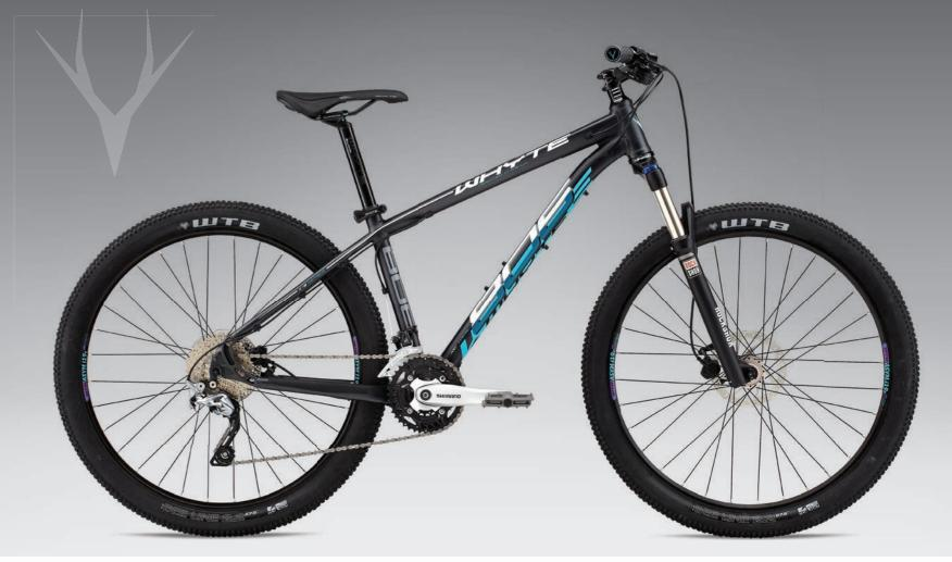
Shimano Deore 3x10spd drivetrain / Compact geometry and sizing down to XS for smaller riders / Adjustable air-sprung RockShox Recon Silver suspension fork X8 PERFORMANCE HARDTAIL 650b/27.5"
