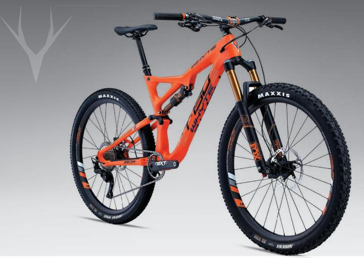
SCR Carbon/Alloy frame with symmetrical chainstays for increased stiffness / Shimano XT/RaceFace 11-speed drivetrain / Fox Factory 34 fork, Factory DPS rear shock and Reverb Stealth seatpost
