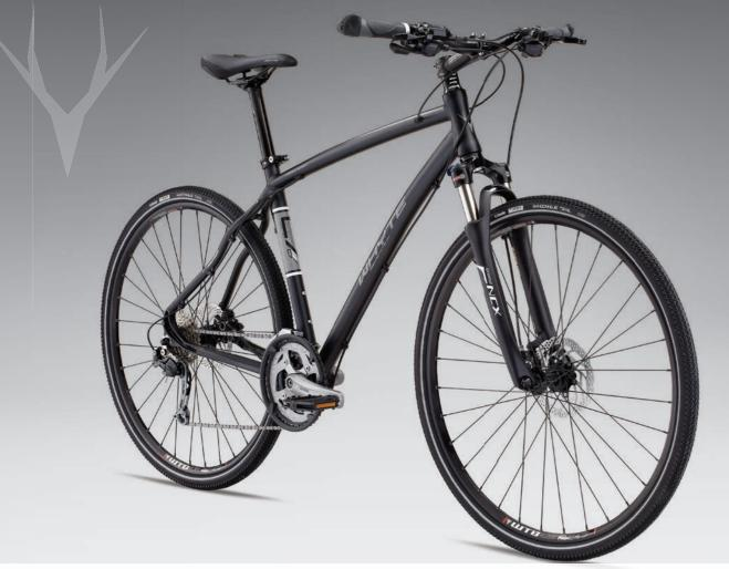
${\tt SR}\ {\tt Suntour}\ {\tt suspension}\ {\tt fork}\ {\tt with}\ {\tt Hydro}\ {\tt lockout}\ {\tt /}\ {\tt Powerful}\ {\tt Shimano}\ {\tt disc}\ {\tt brakes}\ {\tt /}\ {\tt Lightweight}\ {\tt aluminium}\ {\tt frame}$
