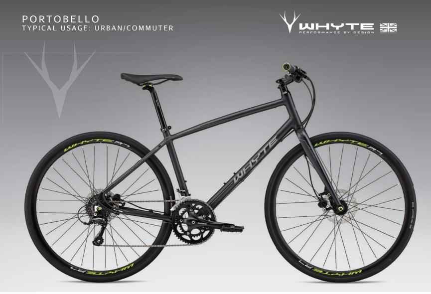
Lightweight aluminium frame with carbon fibre fork / Shimano 2x9spd drivetrain / Vittoria Zaffiro Pro with puncture protection
