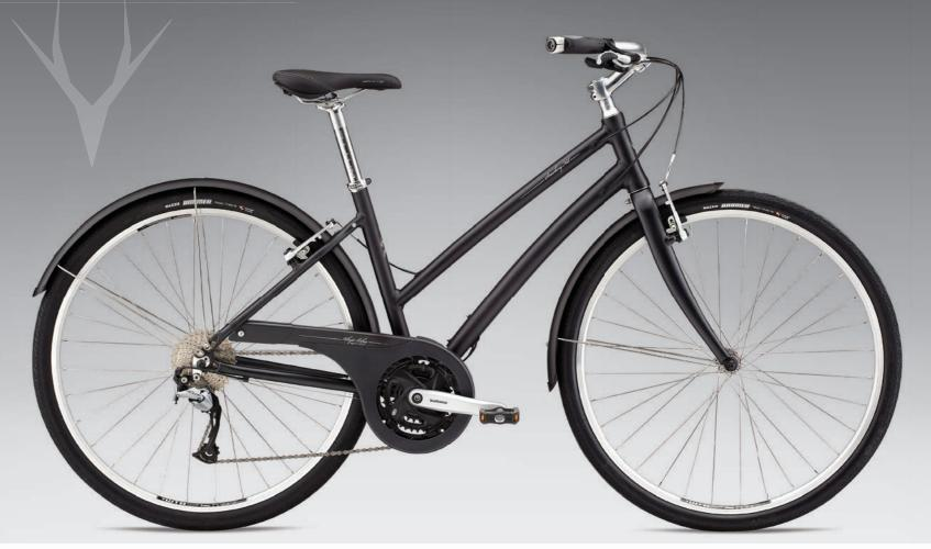
Full-length mud-guards / Shimano 3x10spd drivetrain / Full chainguard / Powerful V-brakes / Lightweight and comfortable Whyte saddle
