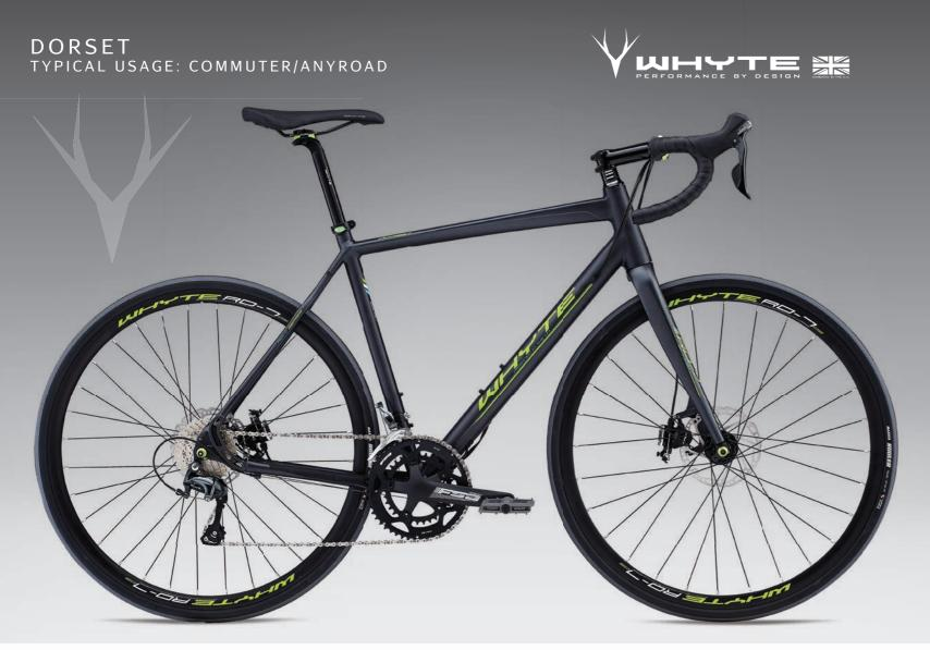
Disc-specific aluminium frame with carbon fibre fork / TRP HyRd mechanical/hydraulic disc brakes / Shimano Tiagra 10spd compact gearing with wide range rear cassette / Internal fork routing
