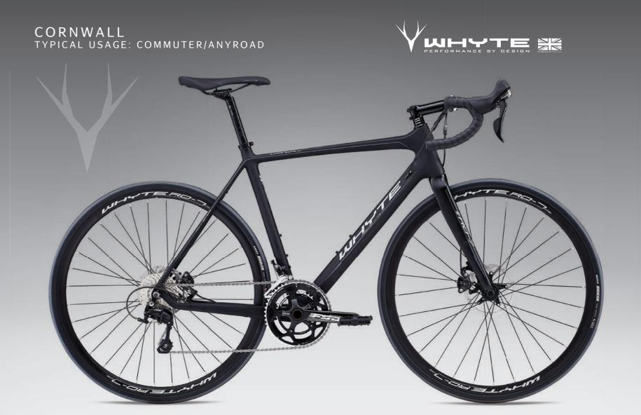
Uni-directional multi-monocoque carbon frame with carbon fork / Shimano 105 fully hydraulic disc brakes / Shimano 105 drivetrain / Internal fork routing RD7 CARBON ROAD DISC
