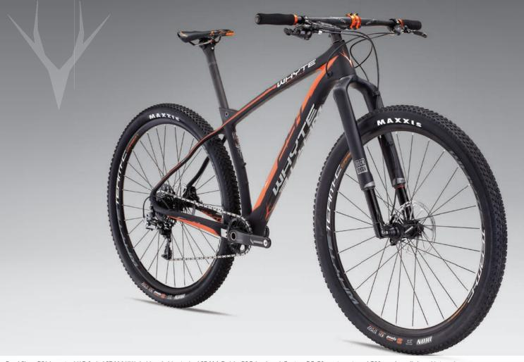
RockShox RS1 inverted XC fork / SRAM XX1 1x11spd drivetrain / SRAM Guide RSC brakes / Easton EC-70 seat post and 720mm handlebar / Intergrip
