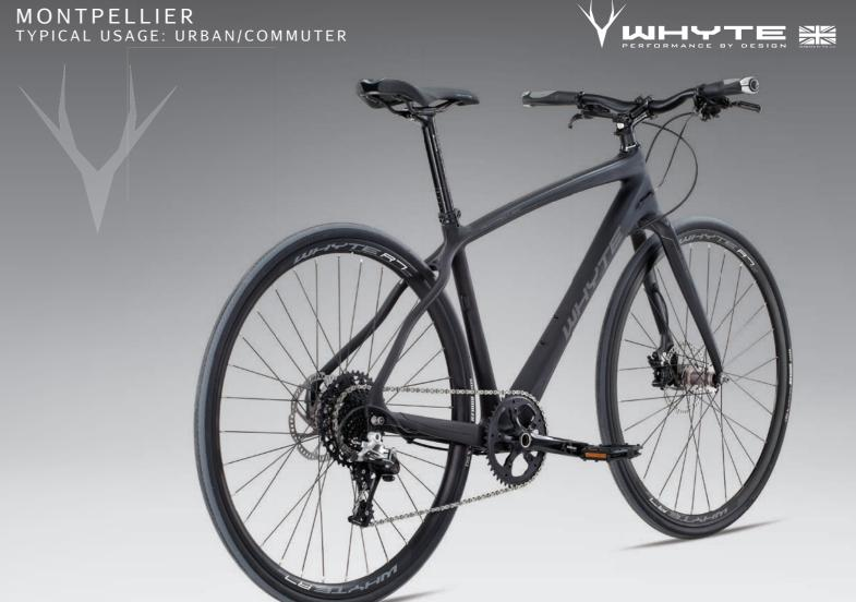
Full carbon frame is 300g lighter than aluminium / SRAM Rival 1, 1 by 11 groupset/ lightweight carbon fibre fork with internal cable routing  $R7\ FAST\ URBAN\ SERIES$
