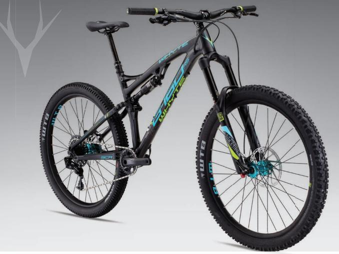
RockShox Pike RC fork DebonAir shock and Reverb Stealth seatpost / 29mm wide WTB TCS tubeless ready rims and tyres / SRAM X-1 11-speed drivetrain with SRAM Guide R brakes GRAVITY ENDURO 650b/27.5"
