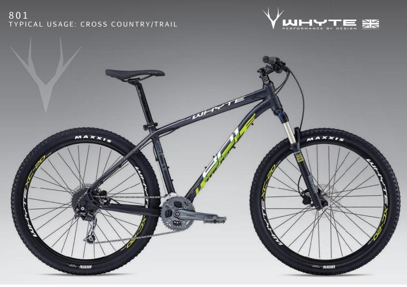
Shimano 3x9spd drivetrain provides gears for all terrain / Maxxis Ikon tyres roll fast and grip well / RockShox 30 Silver fork with TurnKey lockout and Solo Air  $X8\ PERFORMANCE\ HARDTAIL\ 650b/27.5"$
