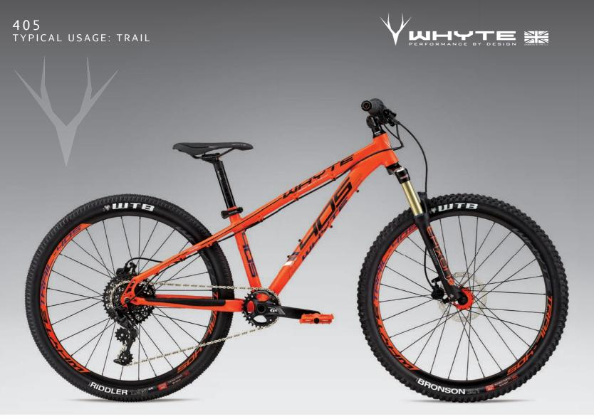
SRAM GX 1 by 11 drivetrain with GX GripShift shifter and/SR Suntour Epicon fork with adjustable air spring to tune to rider weight / Tailored front and rear tyres to exploit every ounce of grip and performance
