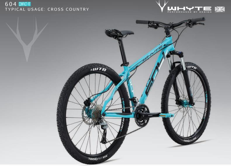
Lightweight aluminium frame with compact geometry for smaller riders / 100mm travel SR Suntour suspension fork / Tektro Auriga hydraulic disc brakes with short reach levers  $X6\ SPORTS\ HARDTAIL\ 650b/27.5"$
