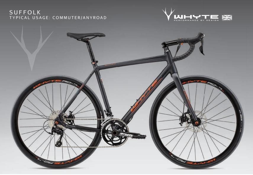
Shimano 105 11-speed drivetrain / Powerful TRP HyRd mechanical/hydraulic disc brakes / Carbon fork with alloy steerer tube / Internal fork routing RD7 DISK ROAD
