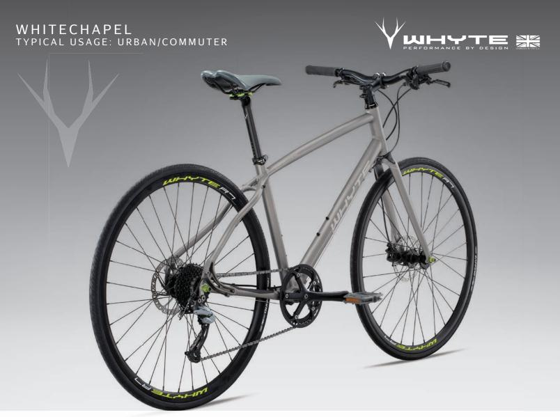
Tektro hydraulic disc brakes / 1x9spd Shimano drivetrain for urban simplicity / Lightweight aluminium frame
