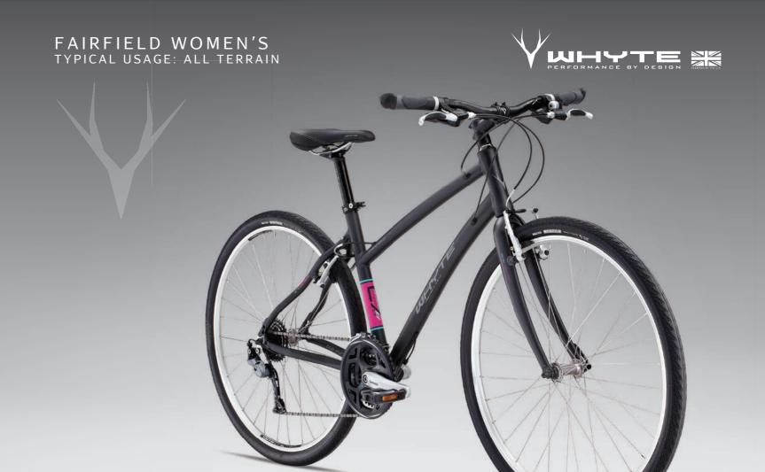
Partially dropped top tube is stronger than a fully dropped frame / Maxxis Roamer tyres with puncture protection / Wide-ratio Shimano gearing C7 ALL TERRAIN WOMEN'S
