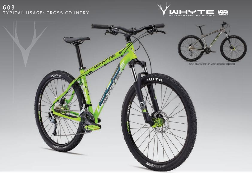
Lightweight aluminium frame with internal cable routing / SR Suntour suspension with lockout feature / Tektro Auriga hydraulic disc brakes  $X6\ SPORTS\ HARDTAIL\ 650b/27.5"$
