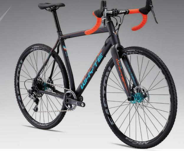
SRAM Force 1 1x11spd drivetrain and hydraulic disc brakes / Easton ARC-24 tubeless rims with Maxxis TR tyres / Whyte CX carbon disc fork with 15mm Axle and internal cable routing
