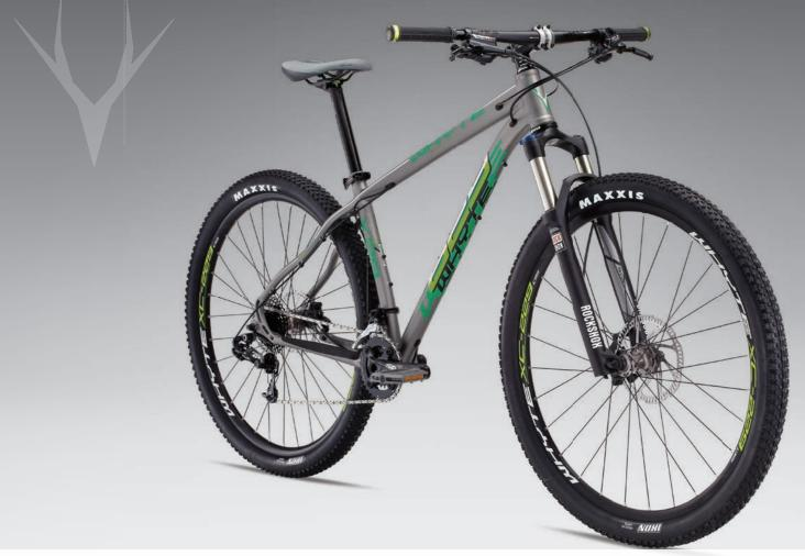
SRAM GX 2x10spd drivetrain / RockShox Recon Silver TK air-sprung fork with 100mm of travel / Fast rolling Maxxis Ikon tyres
