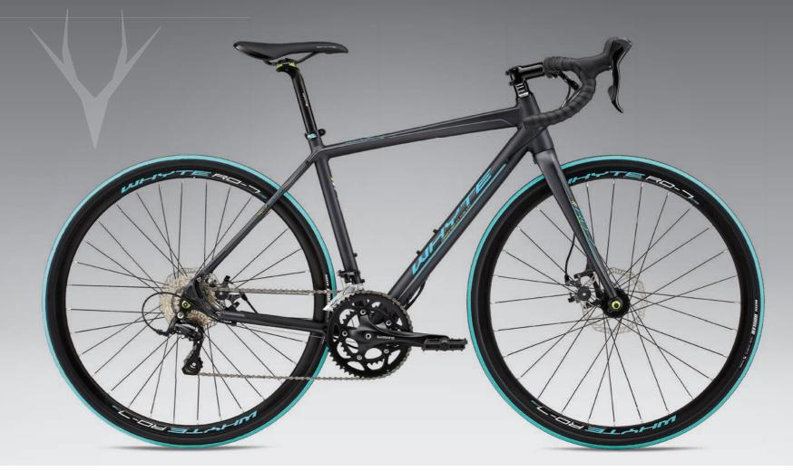
Lightweight disc-specific aluminium frame with alloy fork / Shimano 9spd compact gearing with wide range rear cassette / Powerful mechanical disc brakes / Internal fork routing
