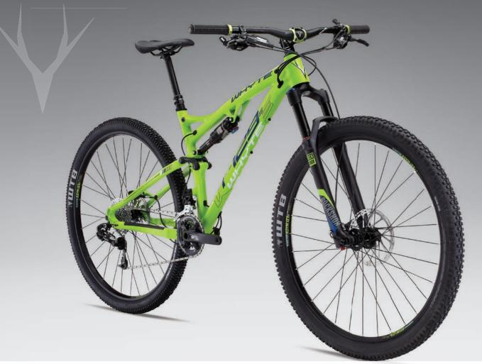
RockShox Reverb Stealth seatpost, Revelation RL fork and Monarch DebonAir shock / SRAM GX 2x10spd drivetrain/ WTB tubeless-ready offset rims and tyres
