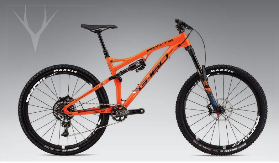
SRAM Rail 40 wheels with tubeless ready Maxxis High Roller II/Minion SS tyres / SRAM XX1/XO drivetrain with SRAM Guide RSC brakes / Oversized RaceFace 35mm X 800mm carbon bars and Easton Haven alloy 32mm long stem
