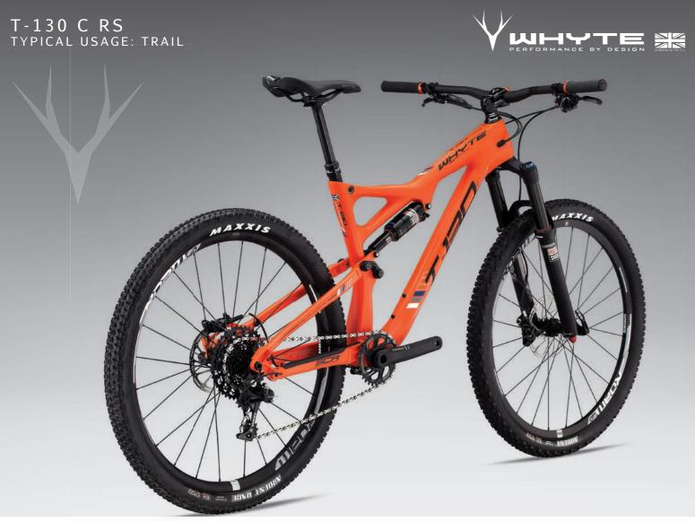
SCR Carbon/Alloy frame with symmetrical chainstays for increased stiffness / SRAM X-1/X-0 11-speed drivetrain / RockShox Pike Boost fork, Monarch DebonAir shock and Reverb Stealth seatpost
