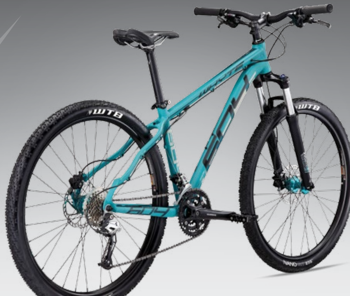
Lightweight aluminium frame with compact geometry for shorter riders / 100mm travel SR Suntour suspension fork / Tektro Auriga hydraulic disc brakes X-6 SPORTS HARDTAIL 650B / 27.5"
