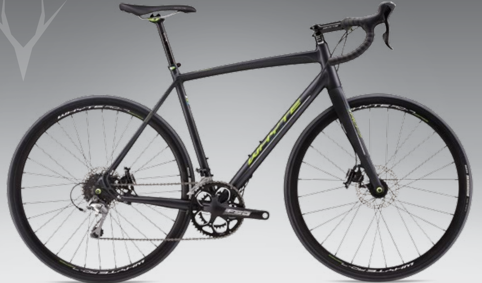
Disc-specific aluminium frame with carbon fibre fork / TRP HyRd mechanical/hydraulic disc brakes / Shimano Sora 9spd compact gearing with wide range rear cassette RD-7 ROAD DISC
